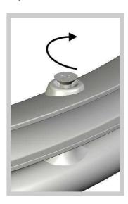
Place the bolts and the bolt caps (x6) through the Loopwheel and down into the push rim. Screw the bolts into place using a 'posi-drive' screw driver, to a torque setting of 5 N/mm. (Option to thread lock the bolts in place)
