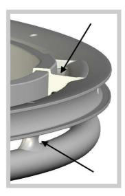
Place the Loopwheel onto the 'push rim spacers', making sure the wheel is orientated so that the 'rib' on the 'rim connector' is on the opposite side to the push rim.
