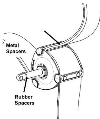
STEP 11: Replace the wheels onto the chair.
