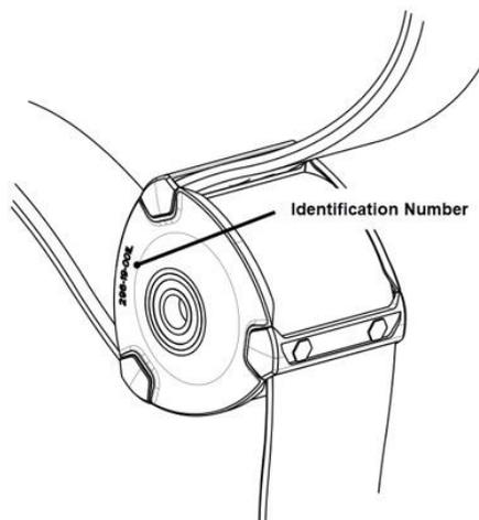
STEP 6: Push one axle into each Loopwheel™ from the other, outward facing side of the wheel.
