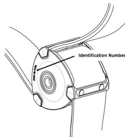
STEP 6: Push one axle into each Loopwheel™ from the outward facing side of the wheel.
