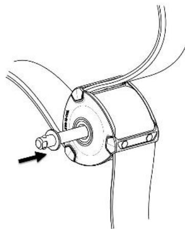
STEP 10: Secure the steel spacers in place by sliding the rubber washer onto the Loopwheel™ axle.
