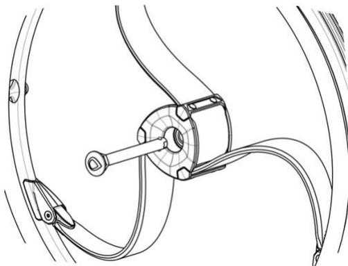
STEP 7: Insert the axle (with the wheel on it) into the axle housing on your wheelchair, one side at a time. R on right hand side; L on left hand side.
