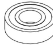
The bearings are fixed into the wheel hub.
