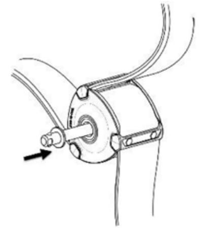
STEP 10: Secure the steel spacers in place by sliding the rubber washer onto the Loopwheel™ axle.
