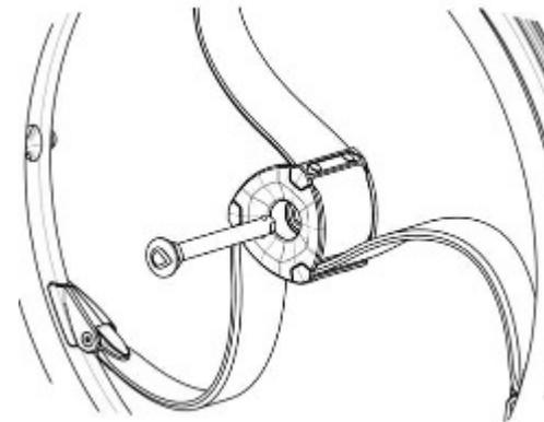
STEP 7. Insert the axle (with the wheel on it) into the axle housing on your wheelchair, one side at a time.
