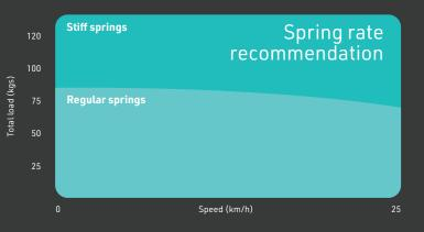
Loopwheels Extreme is available in 2 spring strengths -Regular Springs and Stiff Springs. Use the chart above to estimate the most usual higher speed on the wheels and the fully-loaded weight of the chair.
