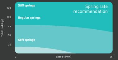
**Loopwheels Urban** is available in 3 spring strengths – **Soft springs, Regular springs** and **Stiff springs**. Use the chart above to estimate the most usual higher speed on the wheels and the fully-loaded weight of the chair.
